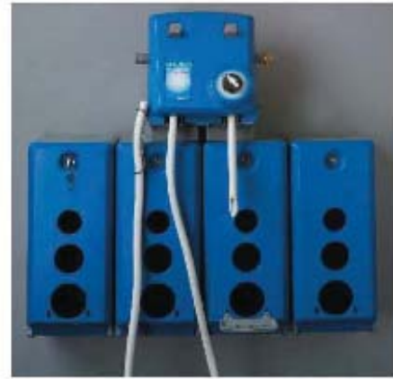
830GAP-Q1G 1 gpm four chemical Dial-A-Blend (4 liters/minute) 4 gpm single product bucket fill (16 liters/minute) Four 1 gallon/5 liter locking enclosures
